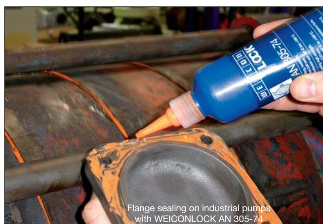
Flange sealing on industrial pumps with WEICONLOCK AN 305-74
