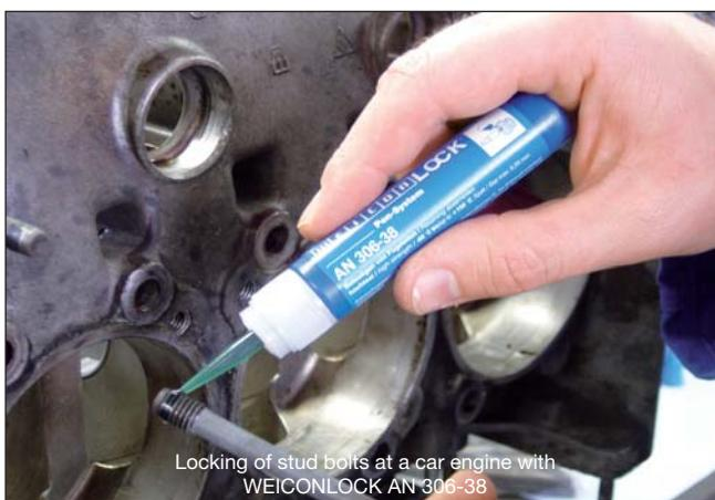
Locking of stud bolts at a car engine with WEICONLOCK AN 306-38
