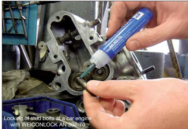
WEICONLOCK products are high quality anaerobic adhesives and sealants on the basis of special methacrylate resins, especially made for economical threadlocking, retaining and sealing of threaded, cylindrical and pipe assemblies.
