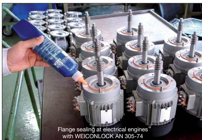
Flange sealing at electrical engines\* with WEICONLOCK AN 305-74
