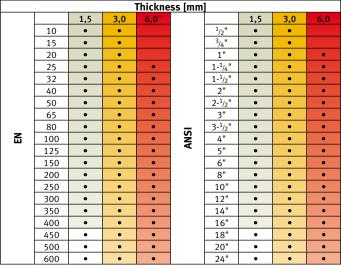
recommended thickness 1.5 for steel piping
