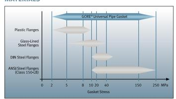
Due to the very low minimum gasket load required, GORE® Universal Pipe Gasket (Style 800) seals all typical types of flanges.
