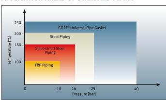
95% of all chemical processes run at temperatures of up to 200 °C and 25 bar. **GORE® Universal Pipe Gasket** (Style 800) offers the highest performing ePTFE gasket and largest operating zone.
