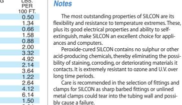
^SILCON may be low pressure steam sterilized in-line or autoclaved at up to 250°F in a normal autoclaving cycle. However, if exposed to repeated steam sterilization or long-term high temperature or pressure, silicone will eventually relax and become gummy. It should then be replaced.
